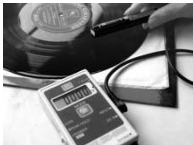
Measuring charge with a static charge tester.
